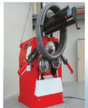
Pipe rolling machines
